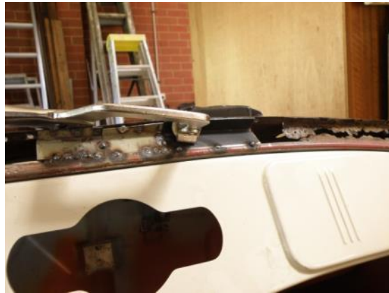
Figure 11. Commencing rewelding new metal below the wind screen.
