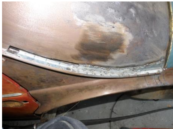
Figure 8. Partially repaired rusted roof and gutter.
