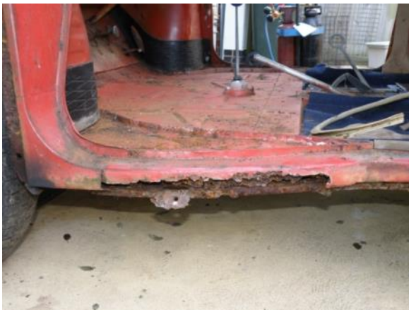
Figure 5. Rust in the body below the front door (neither side was better).
