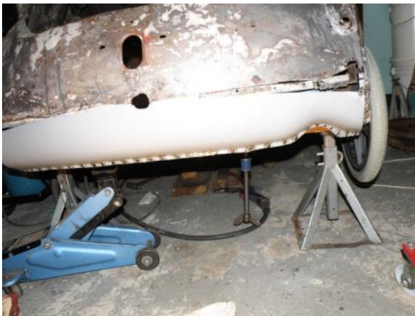
Figure 10. Welding in the replacement rear end.
