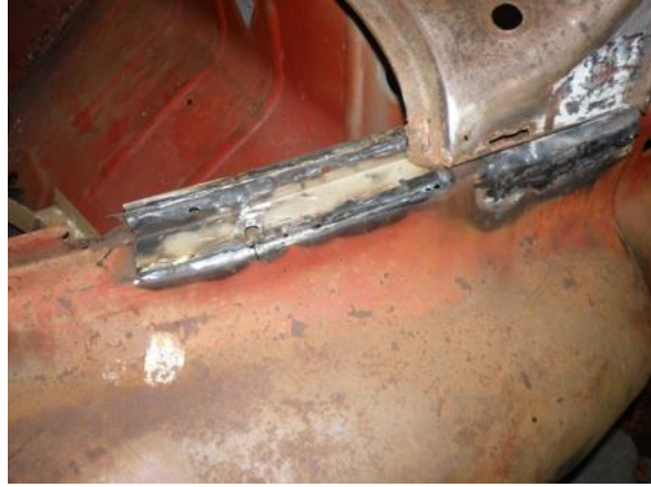
Figure 7. A partially repaired front mudguard.
