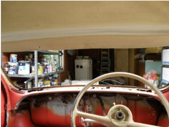
Figure 4. Rust holes below windscreen.
