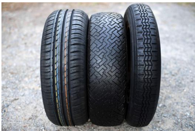
Evolution of rear tyres: (current) 185/60-14 Continental EcoContact3, CN36 SM & X
