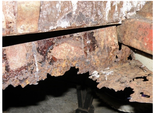
Figure 3. The boot with the bottom fully removed.
