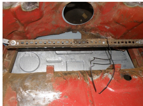
Figure 6. The boot finally welded in position.
