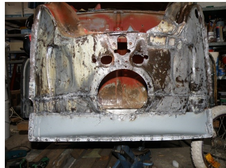
Figure 9. Shows the trimmed new front face partially welded along with the two pieces that I had previously removed.
