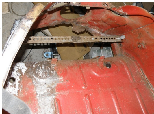
Figure 4 shows the new boot bottom in place prior to spot welding it from underneath the car.
