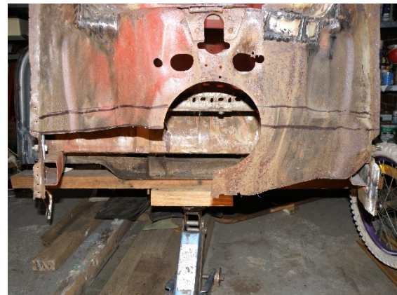
Figure 8. Right side of front face removed before fitting the new front face.
