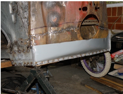
Figure 9. Shows the trimmed new front face partially welded along with the two pieces that I had previously removed.
