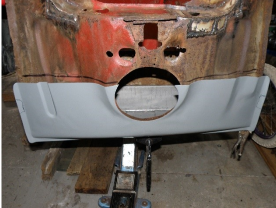
Figure 7. The new front to be welded into the body to replace the rusted section.
