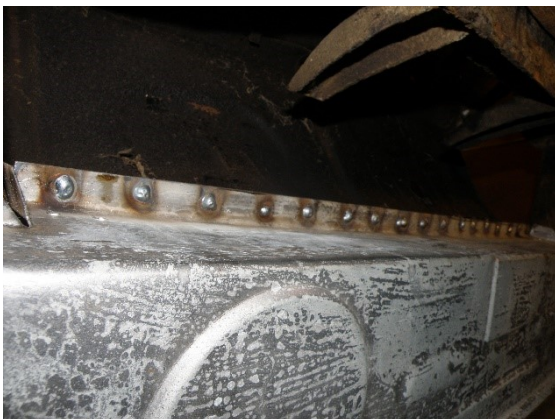
Figure 5. The initial spot welds to hold the boot in position.
