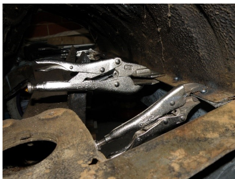
Figure 3. The boot with the bottom fully removed.
