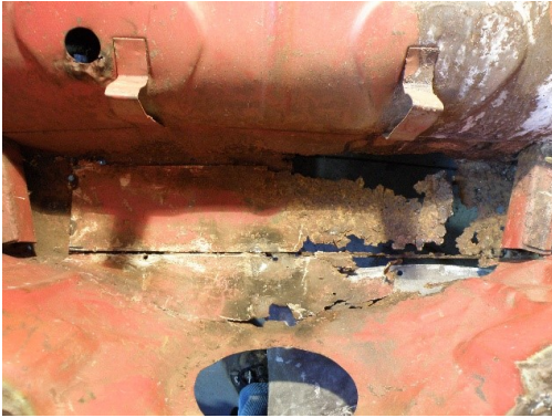
Figure 1. The rusted boot bottom and front face of the car.
