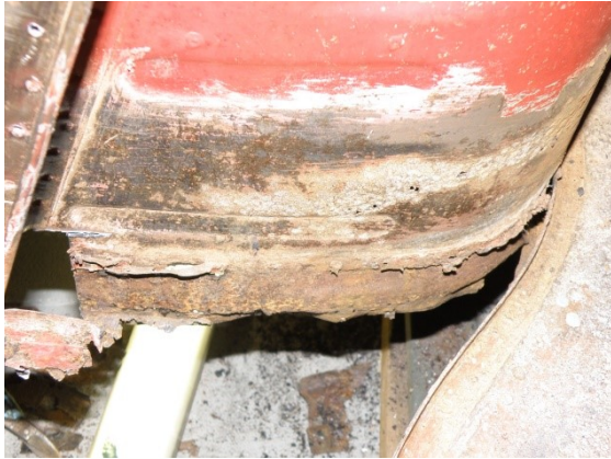
Figure 1. Rusty wheel arch from inside the car.
