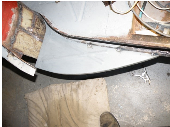
Figure 5. The bottom triangle tack welded in position.
