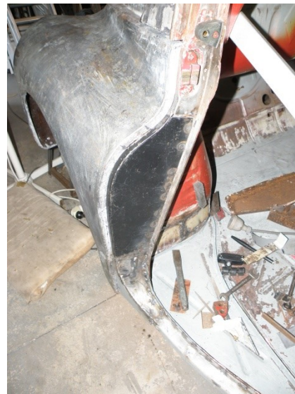
Figure 10. Front door jamb and front door corner welded in place.
