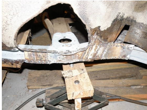
Figure 4. Spot welded cover on front section of C- frame.
