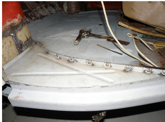
Figure 6. The top triangle spot welded in position.
