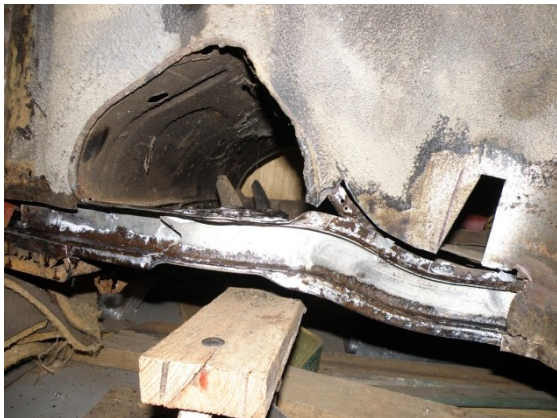
Figure 3. C-frame after phosphoric acid treatment.
