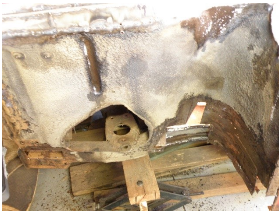
Figure 2. Rusty metal covering the C-frame.
