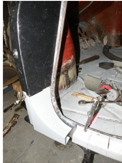
Figure 9. Trial fitting of front door jamb and front door corner.
